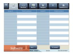
The 7.8 inch LED touch screen is used for management of smear and reagent, performing basic operation and maintenance.
