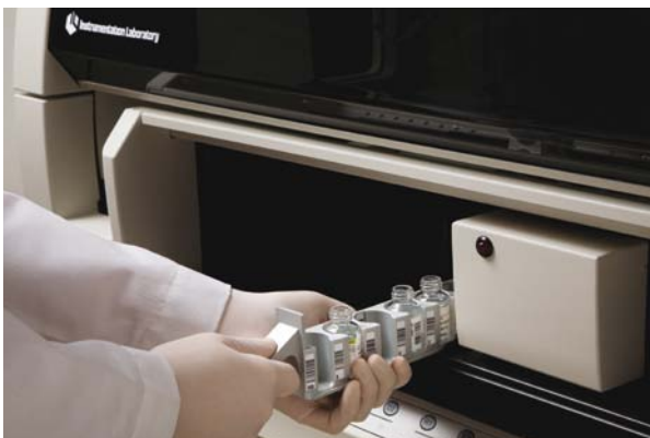
Onboard barcode reader allows real-time reagent management.
